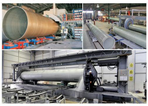
As regards the GRP pipes consist of advanced engineering of fiberglass and resin with specific compositions, the manufacturer could achieve the pipes with desired characteristics choosing correct composition of material and process.
